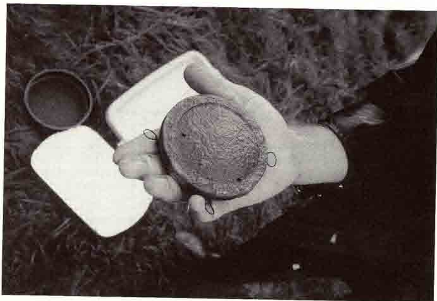
Fig. 1. Photograph of a nutrient diffusing substrate retrieved from river after 5 weeks of incubation.
